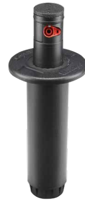
G75B Pop-up height: 8 cm Overall height: 23 cm Flange diameter: 12cm Female Inlet: 1/4" ACME
