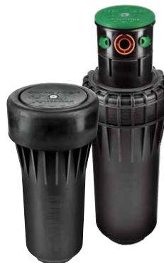
ST-90* Overall height: 29 cm Pop-up height: 8 cm Diameter: 14 cm Inlet size: 1½" BSP * not for use with the ST Vault
