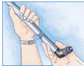
Assembling Poly Pipe: 1. Place clamp over pipe, then insert barb fitting.
