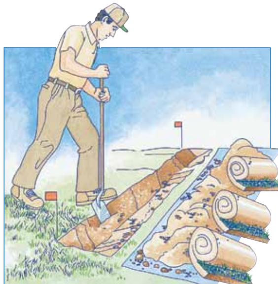
First lay down tarps and remove sod, then dig trenches 25 cm to 30 cm deep for the main line. Trench 15 cm to 20 cm for lateral lines.
