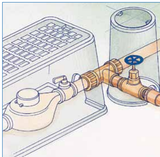
P.O.C. to city water supply: Use a brass compression tee to connect your sprinkler system to the household water supply.
